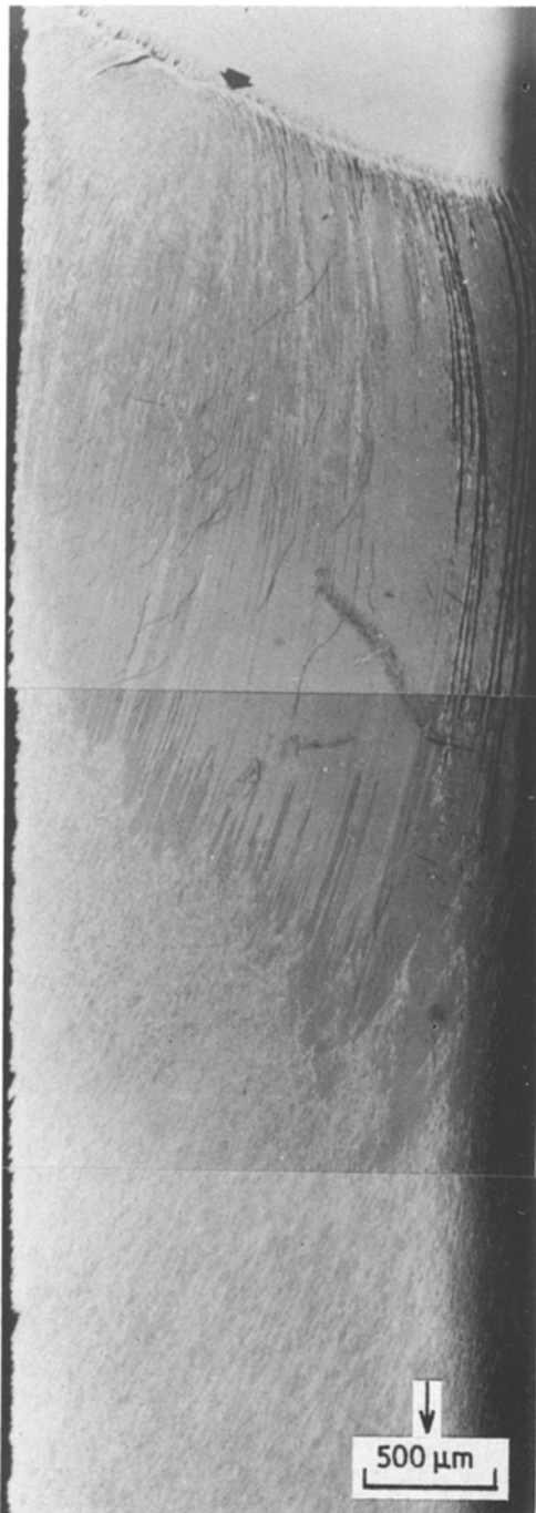
Figure 13 828/TEA: Type II fracture surface, \Delta = 5 \times 10^{-3} \text{ cm min}^{-1} (transmitted light).
